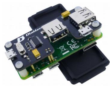
USB SHOE for Raspberry Pi Zero 1.2 gives you Wi-Fi through USB ports without solder anything and keeping the dimensions of the Zero.
